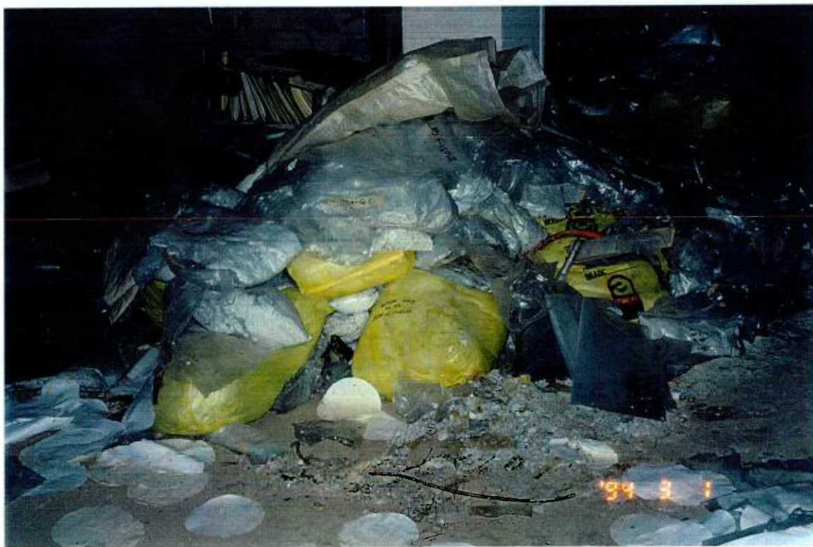
Processed asbestos fibre in broken plastic packaging.
